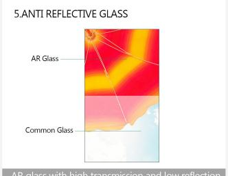
AR glass with high transmission and low reflection Almost 100% of UV is blocked and IR transmission significantly reduced.
